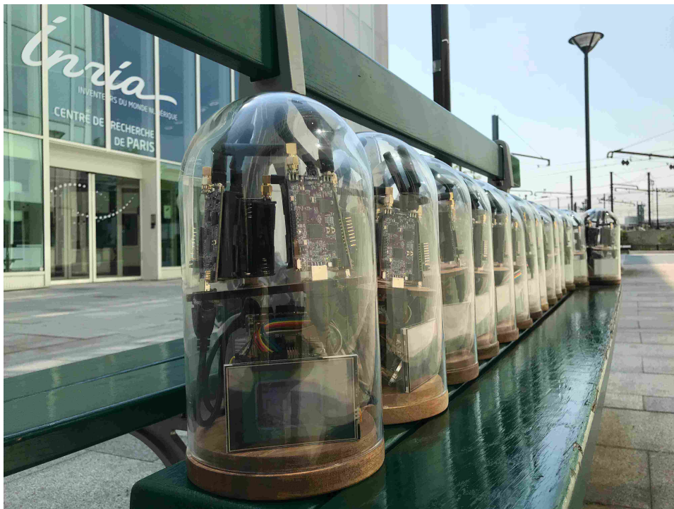
Figure 7.2: The Inria-Paris OpenTestBed before deployment. 20 OtBox contain a total of 80 OpenMote B boards.
