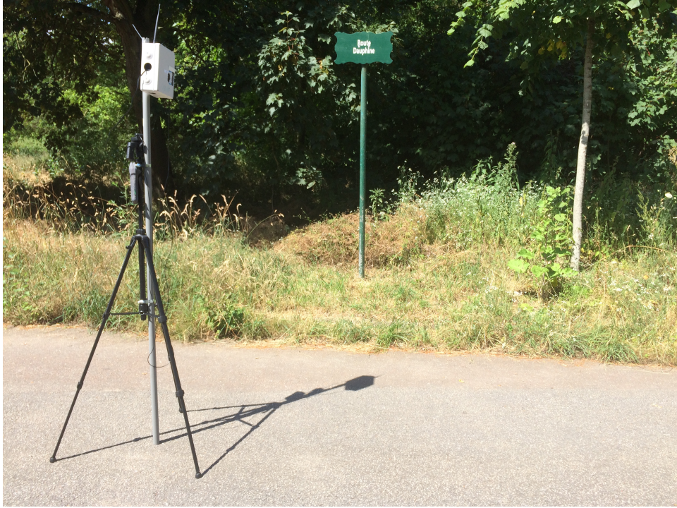
Figure 3.2: A node in a field experiment. Nodes are mounted on a 1.8 m tripod.
