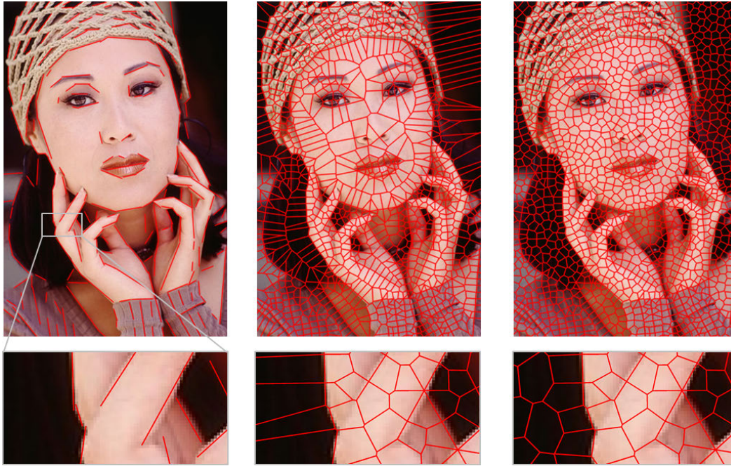
Figure 2.2: Overview of the polygonal partitioning. Left: line-segments are first extracted from the input image, and consolidated to bring spatial coherence (Section 2.4). Middle: an initial Voronoi partition that preserves the line-segments and their junctions is then created by inserting anchors at specific locations (Section 2.5). Right: the Voronoi partition is homogenized by point process (Section 2.6).
