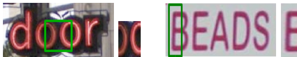
Figure 2.12 – Typical challenges in character detection. (left) Inter-character confusion: A window containing parts of the two o 's is falsely detected as x . (right) Intra-character confusion: A window containing a part of the character B is recognized as E .
