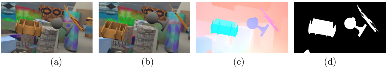
Figure 3.13 – (a,b) Two example frames from a sequence in the FlyingThings3D dataset [108]. The camera is in motion in this scene, along with four independently moving objects. (c) Ground-truth optical flow of (a), which illustrates motion of both foreground objects and background with respect to the next frame (b). (d) Ground-truth segmentation of moving objects in this scene.
