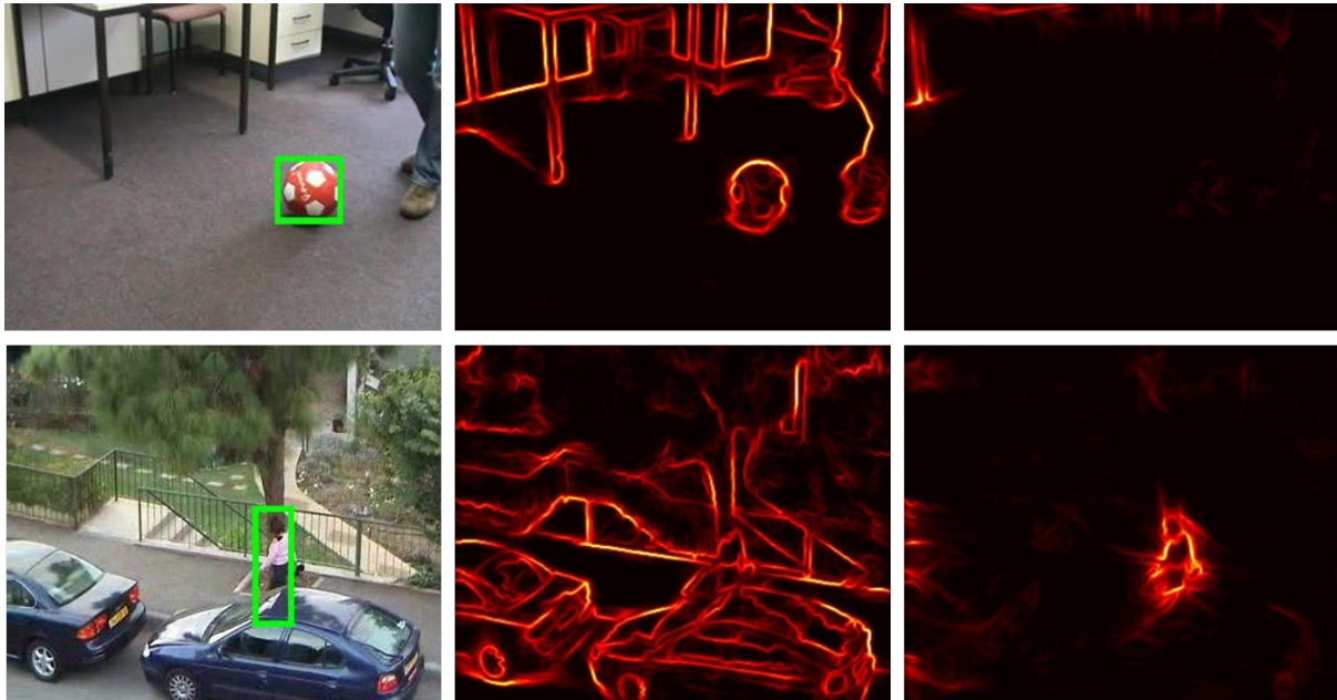
Figure 3.10 – Two examples of edge and motion boundary responses. In each row, from left to right, we show the original image (with the object in a green box), edges and motion boundaries. The edges provide a stronger response in the example in the first row while motion boundaries are more effective in the example in the second row.
