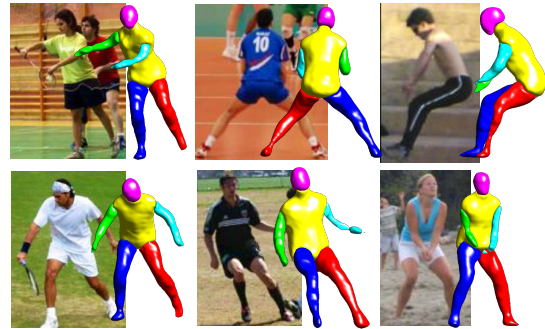
Figure 4-6 – BodyNet is able to directly regress volumetric body parts from a single image on examples from UP.
