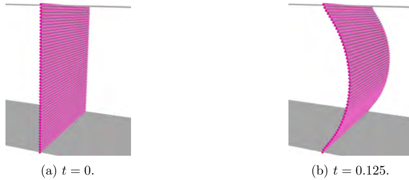
Figure E.5 – Zoom on the fluid and solid meshes at different time instants for the case of the closed valve extended to 3D.
