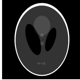
Figure 6.3 – 2D grayscale synthetic phantom of a head where the large ellipse represents the brain while the smaller internal ellipses represent brain features.
