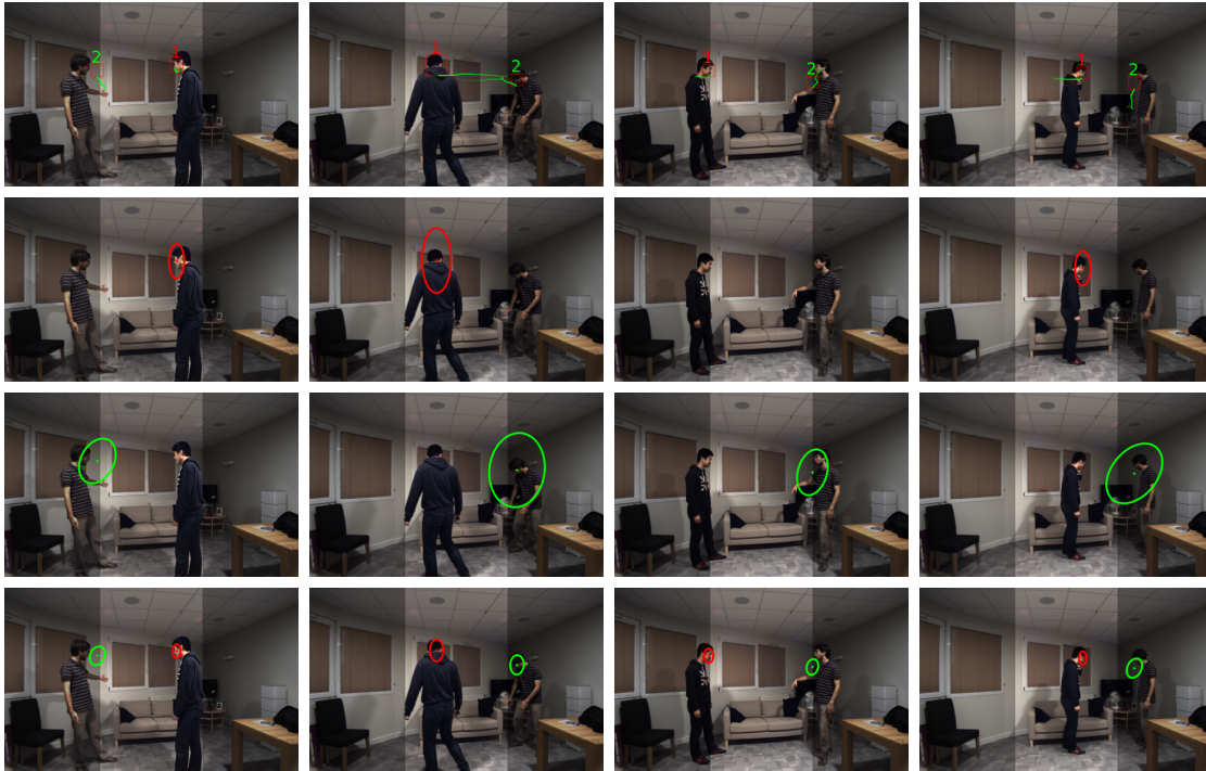
Figure 4.2: Four frames sampled from Seq19-2P-S1M1. The camera field of view is limited to the central strip. Whenever the participants are outside the central strip, the tracker entirely relies on audio observations and on the model’s dynamics.
