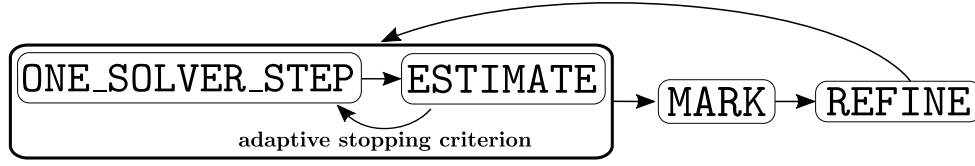
Scheme 2.2: Paradigm of an adaptive loop employing an inexact algebraic solver.
