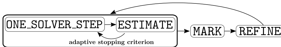
Scheme 2.2: Paradigm of an adaptive loop employing an inexact algebraic solver.
