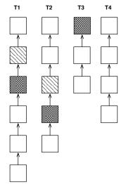
(d) The *gDSU* checks, but the system is not at a Safe Update point because T1 and T2 are still executing methods to be modified.
