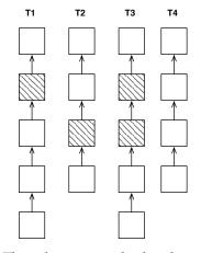
(b) Threads using methods to be modified, in this state the update cannot be applied.
