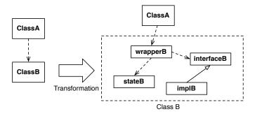
Figure 2.4: Static Transformation performed by DUSC to enable dynamic update of the class.
