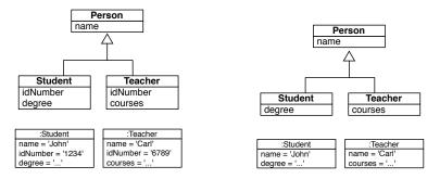
(a) Original State before the refactor- (b) Step 1: Remove subclass instance ing variables
