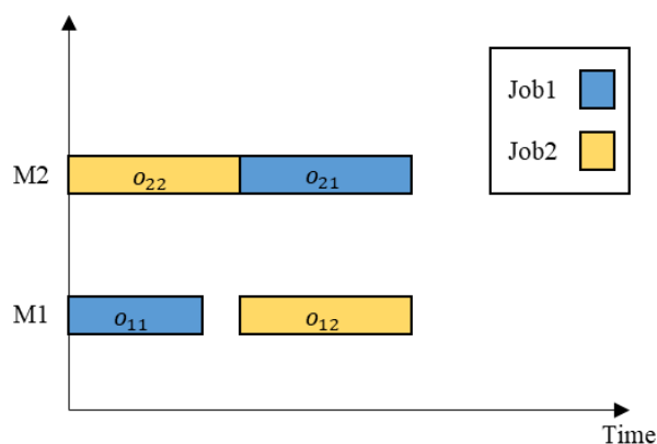
Figure 5-9. Gantt chart of two jobs on two machines.
