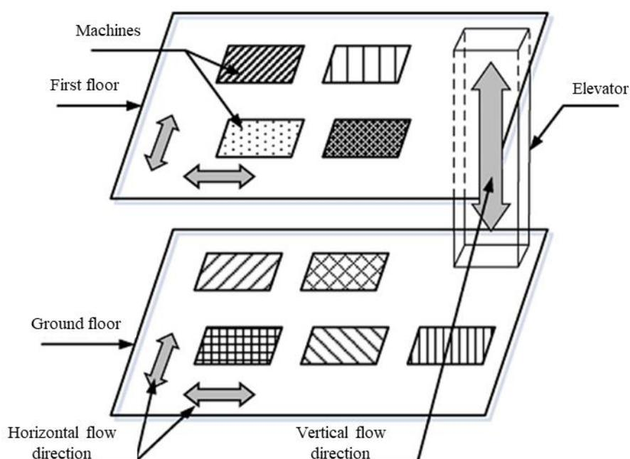
**Figure 3-3.** Multi-floor layout [Drira et al., 2007].
