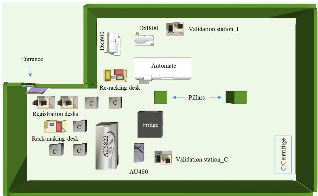
Figure 3-12. Laboratory layout design considering entrance E2.
