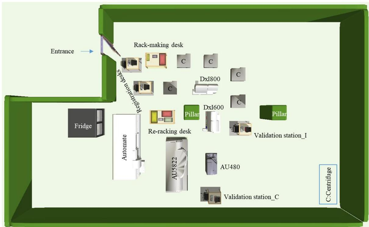
Figure 3-11. Laboratory layout design considering entrance E1.
