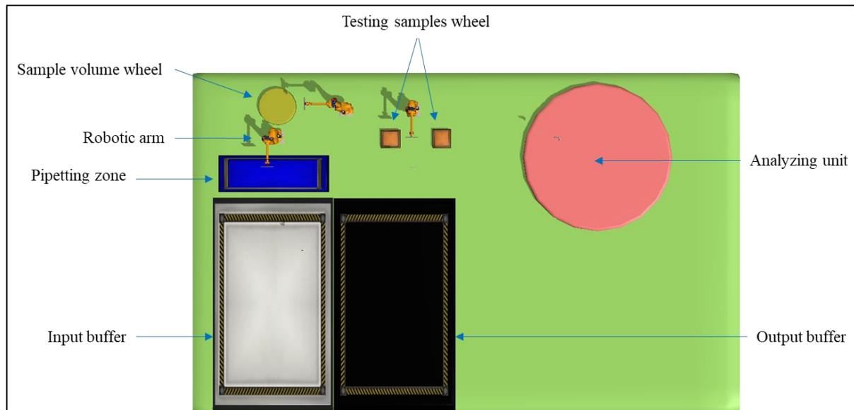
**Figure 6-9.** Components of DxI600 analyzer modeled in FlexSim.
