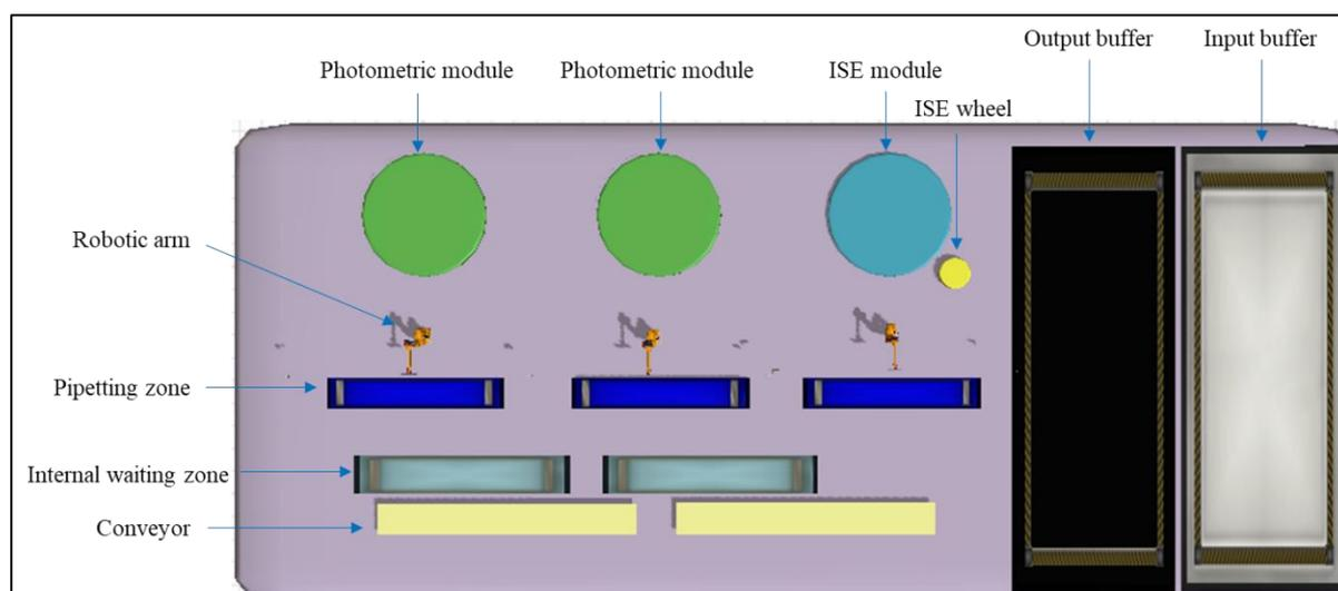
**Figure 6-8.** Components of AU5822 analyzer modeled in FlexSim.
