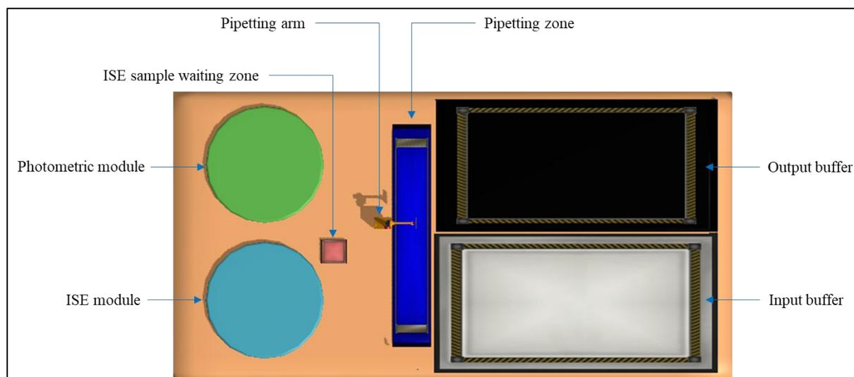
**Figure 6-7.** Components of AU480 analyzer modeled in FlexSim.
