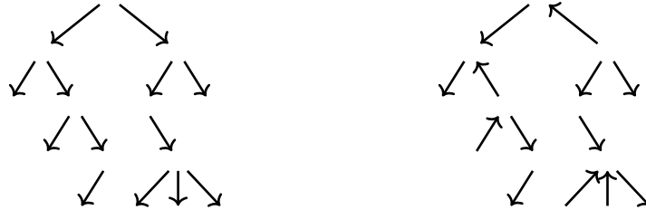
Figure 2 – Examples of unlabeled downward tree (left) and polytree (right)
