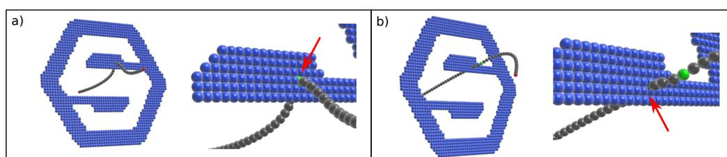
Fig. 8.4 Two types of invalid ART-RRT paths due to: a) atom collision between the string and the obstacles, b) bond collision between a string bond and the obstacles.
