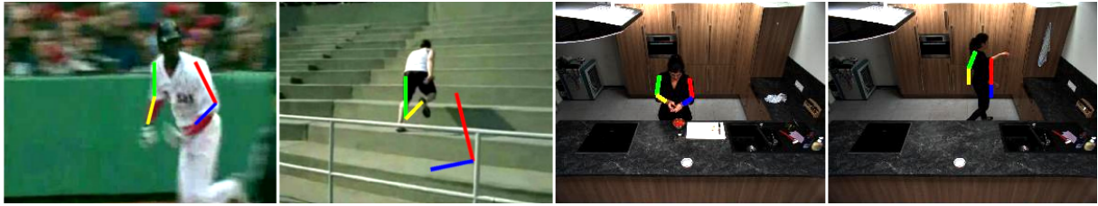
Figure 4.2: Illustration of human pose estimation used in our experiments [Cherian et al., 2014]. Successful examples and failure cases on JHMDB (left two images) and on MPII Cooking Activities (right two images). Only left and right arms are displayed for clarity.
