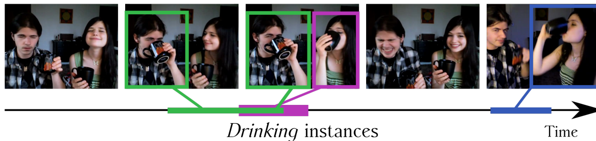
Figure 1.2: Spatio-temporal action localization consists in three sub-tasks: recognizing the action ( drinking ), finding the temporal extent (one horizontal bar for each of the 3 instances) and spatially localizing the actor (person bounding boxes). Examples from the DALY [Weinzaepfel et al., 2016] dataset.
