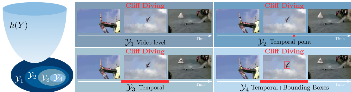
Figure 6.1: A flexible method for handling varying levels of supervision. Our method estimates a matrix Y assigning human tracklets to action labels in training videos by optimizing an objective function h(Y) under constraints \mathcal{Y}_s . Different types of supervision define particular constraints \mathcal{Y}_s and do not affect the form of the objective function. The increasing level of supervision imposes stricter constraints, e.g. \mathcal{Y}_1 \supset \mathcal{Y}_2 \supset \mathcal{Y}_3 \supset \mathcal{Y}_4 as illustrated for the Cliff Diving example above.
