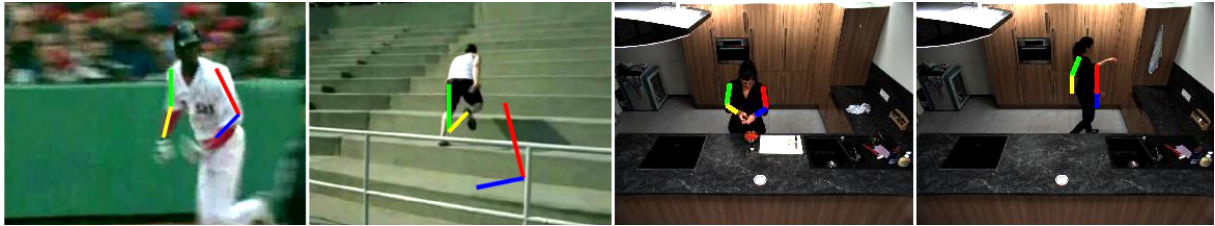
Figure 4.2: Illustration of human pose estimation used in our experiments [Cherian et al., 2014]. Successful examples and failure cases on JHMDB (left two images) and on MPII Cooking Activities (right two images). Only left and right arms are displayed for clarity.
