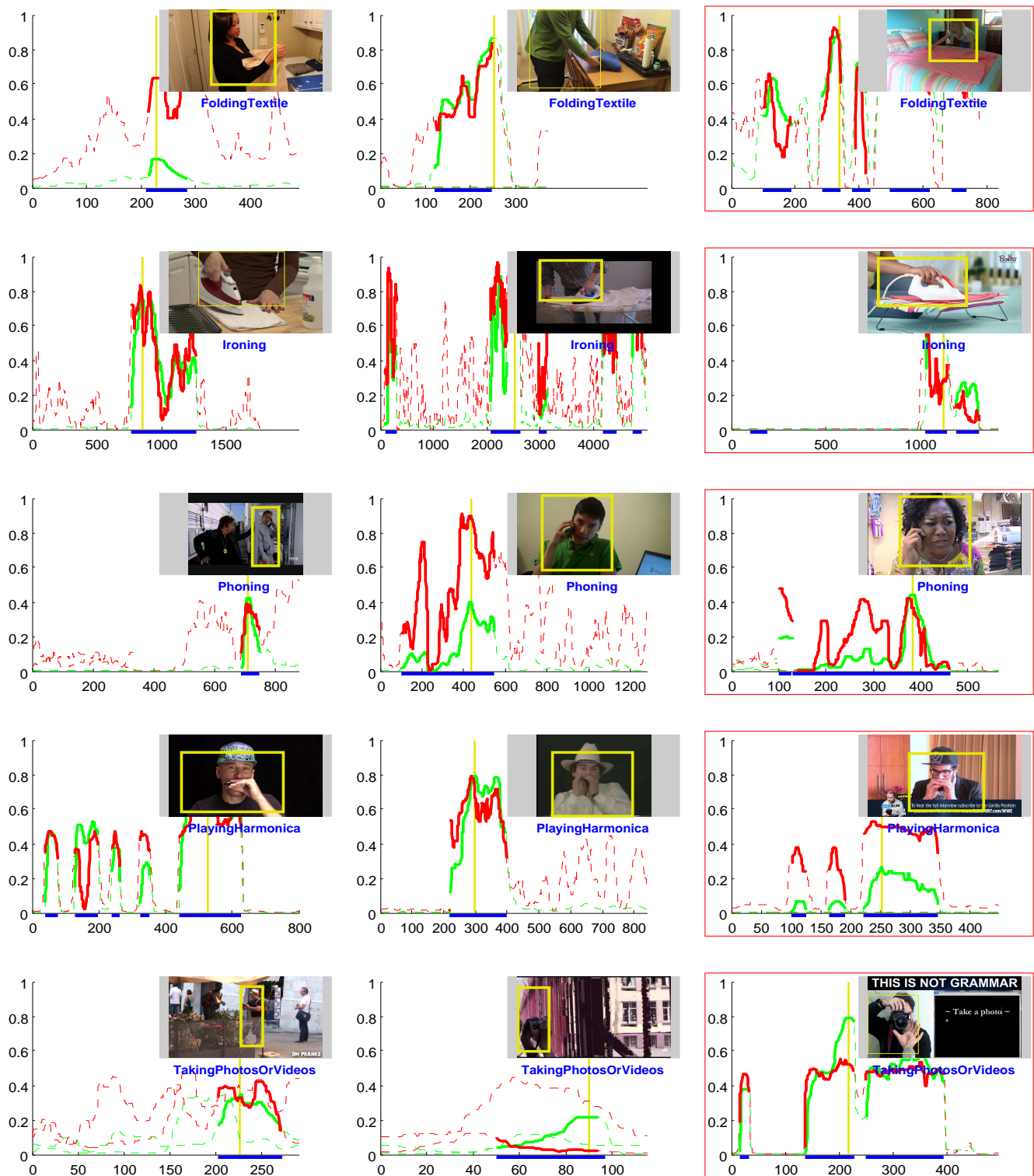
Figure 5.5: Qualitative results for temporal localization on DALY. Each curve represents a human track, green curves correspond to our ReCLNet scores and red ones to scores from CNN features CNN_{RGB+OF} . A bold curve (resp. dashed curve) shows that the track overlaps with more (resp. less) than 0.5 spatial IoU with a ground-truth action. The horizontal blue bar represents the ground-truth time segment. The video frame corresponds to the maximum ReCLNet response (localized at the vertical yellow line) with its associated human detection (yellow box). The last column (red boxes) corresponds to failure cases or examples where our ReCLNet model does not improve temporal localization. Each row corresponds to one action class, namely Folding Textile , Ironing , Phoning , Playing Harmonica and Taking Photos Or Videos . The x-axis represents frame numbers.
