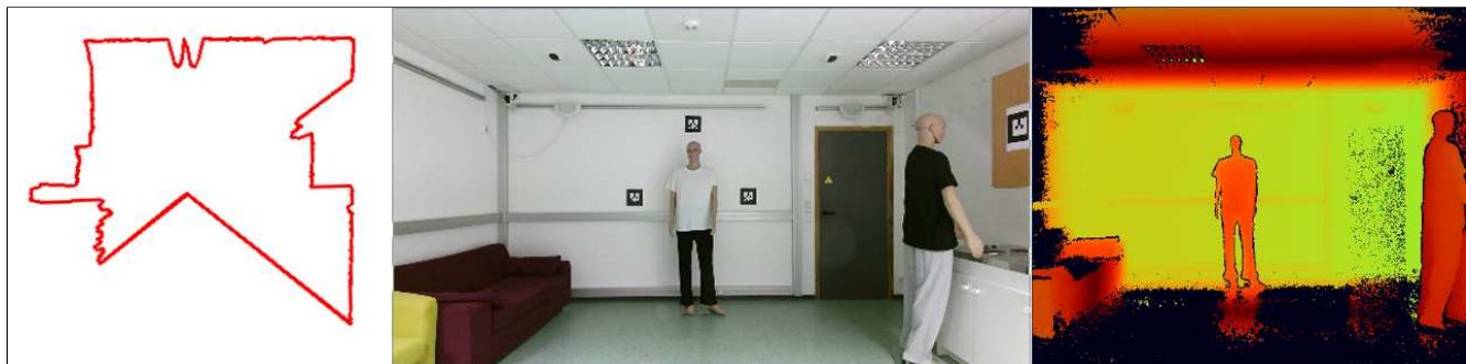
Fig. 8. Robot sensor view. At left, the laser range finder view. In the middle, the RGB stream. Last, the infrared view. The depth view (not on this figure) is aligned with the infrared one.
