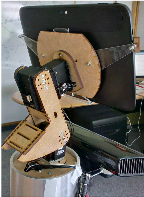
Figure 4: Head mechanical design. The head is built with 4 Dynamixel ® servomotors, laser cutted wood and Plexiglas for the structure and the tablet support. During experimentation, the neck is covered with a textile muff.
