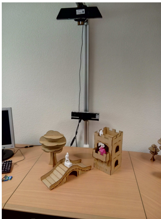
Figure 2: Acquisition setup. There are two Kinect devices: one looking down to follow figurines, one following narrators. The playground area is the table in the middle. Its size in our experiment is 70cm x 70cm.
