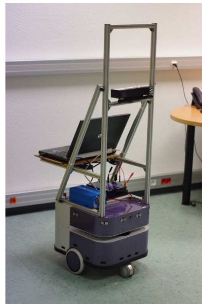
Fig. 1. Robotic platform used for recording: a Robulab10 mobile robot from the Robosoft company. It is equipped with a laser range finder, a Kinect 2.0 and a laptop computer.
