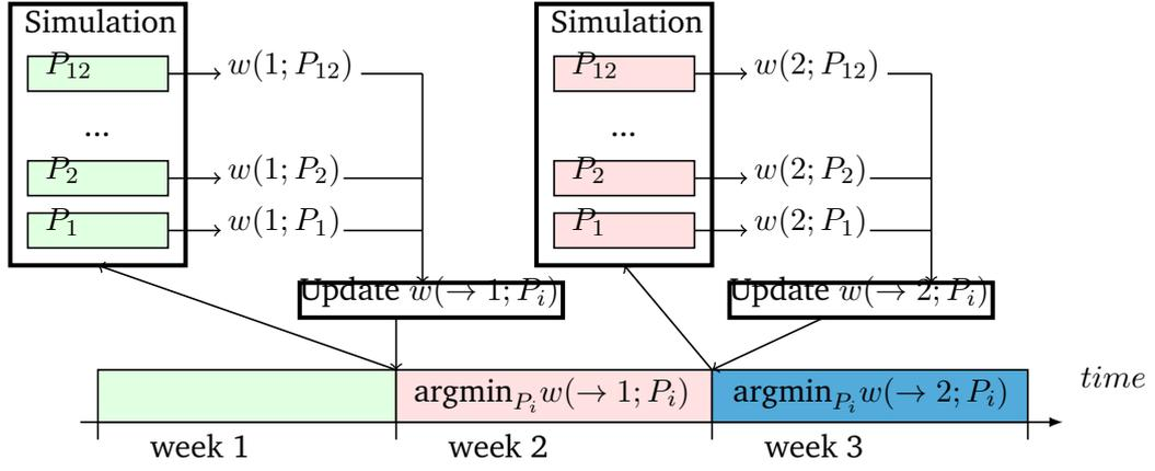
**Fig. 6.2:** Illustration of the online simulation-based strategy. Every week, the workload from the past week is used to run simulations using every reordering policy. The "model"  $w$  is updated according to (6.3) (or (6.6) in the Noisy case from Section 6.3.2) and the policy for the next week is chosen according to (6.4)
