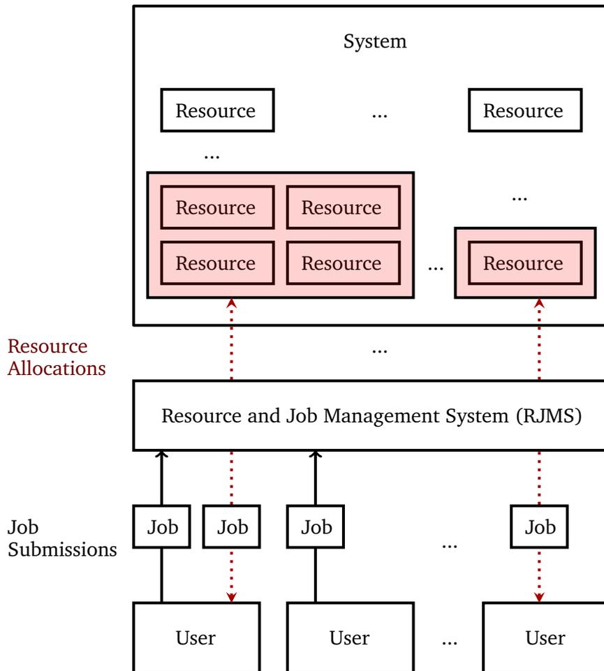
**Fig. 3.1:** Role of the Resource and Job Management System(RJMS). The RJMS manages the platform by giving users restricted access to some resource(s) during some amount of time. Both the resource request and allocated time are the result of the RJMS's decision, which is based on the Job request.
