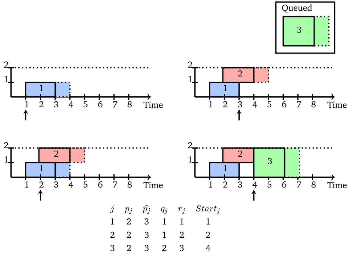
**Fig. 3.4:** Illustration of the scheduling process (time steps 1 to 4) using a simple 'first-come, first serve' policy. This policy waits for space to be available for the oldest job in the waiting queue, and starts it. The characteristics of the three job submissions are given in the table above.
