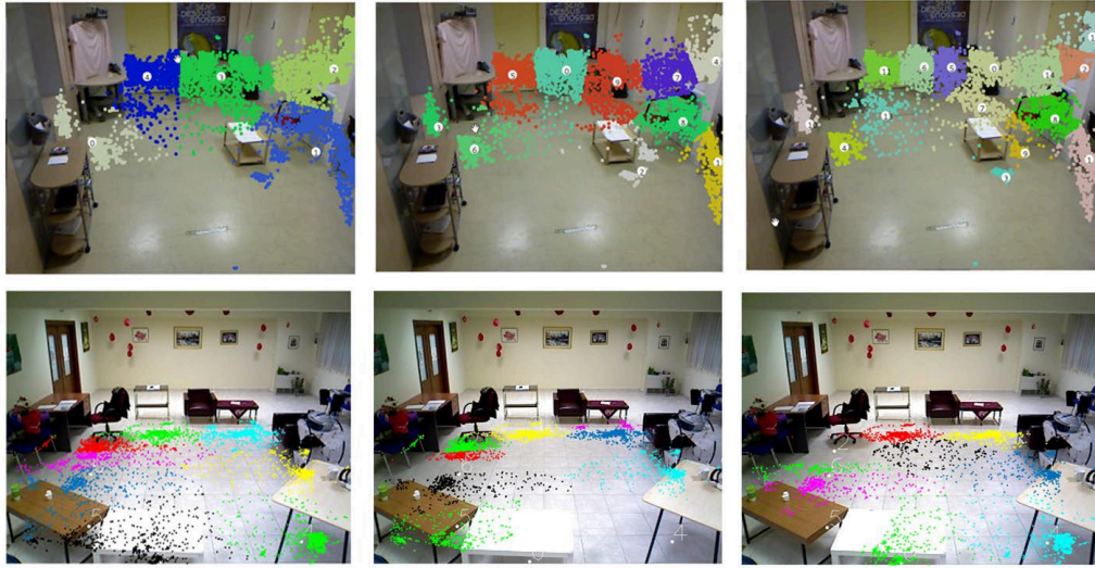
Figure 4.2: Example of k-means clustering using city-block and Euclidean distance measurements. The top row shows samples of CHU Nice dataset clustered using City block distance measure. The number of clusters is set to 5, 10 and 15. Most of the discovered regions can be associated with a semantic activity concept. There are also scene objects that the activity can be associated with. In the below is the GAARDR dataset clustered using Euclidean distance measure.
