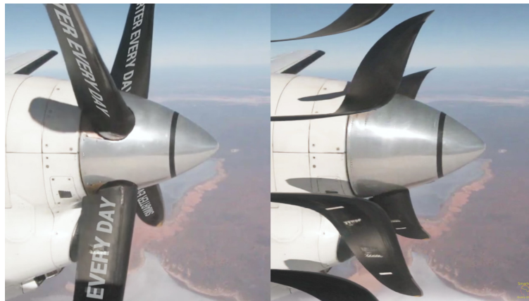
Figure 2.1: On the left, the picture is taken by a global shutter camera. On the right, the camera has a rolling shutter. Source: smartereveryday.com .
