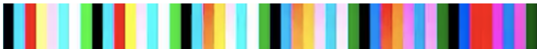
Figure 8.2: The same 8-CSK symbols sent consecutively and repetitively are perceived differently in the picture.
