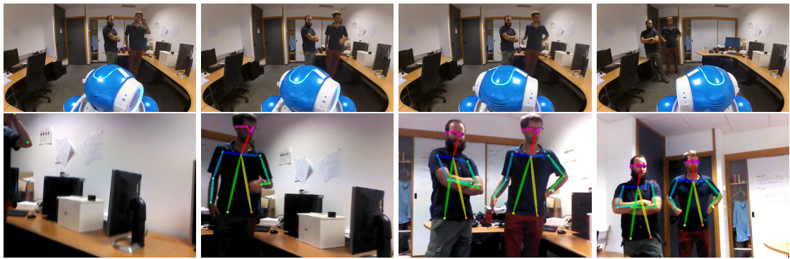
Figure 4.7: Example of a live sequence with two persons. First row shows an overview of the scene, including the participants and the robot. Second row shows the images gathered with the camera mounted onto the robot head. The robot head is first initialized in a position where no face is visible (first column), and the model uses the available landmarks (elbow and wrist) to find the person onto the right (second column). The robot detects the second person by looking around while keeping the first person in its field of view (third column), and gazes the two people walking together (fourth column).
