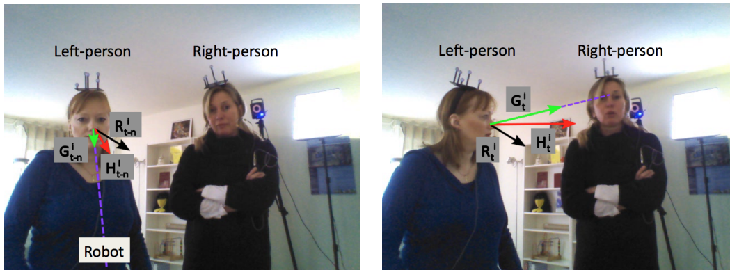
Figure 2.1: This figure illustrates the principle of our method and displays the observed and latent variables associated with a person ( left-person indexed by i ). The two images were grabbed with a camera mounted onto the head of a robot and they correspond to frames t - n (left image) and t (right image), respectively. The following variables are displayed: head orientation (red arrow), \mathbf{H}_{t-n}^i, \mathbf{H}_t^i (observed variables), as well as the latent variables estimated with the proposed method, namely gaze direction (green arrow), \mathbf{G}_{t-n}^i, \mathbf{G}_t^i , VFOA, \mathbf{V}_{t-n}^i, \mathbf{V}_t^i , and head reference orientation (black arrow), \mathbf{R}_{t-n}^i, \mathbf{R}_t^i (that coincides with upper-body orientation). In this example left-person gazes towards the robot at t - n , then turns her head to eventually gaze towards right-person at t , hence her VFOA switches from \mathbf{V}_{t-n}^i = \text{robot} to \mathbf{V}_t^i = \text{right-person} .
