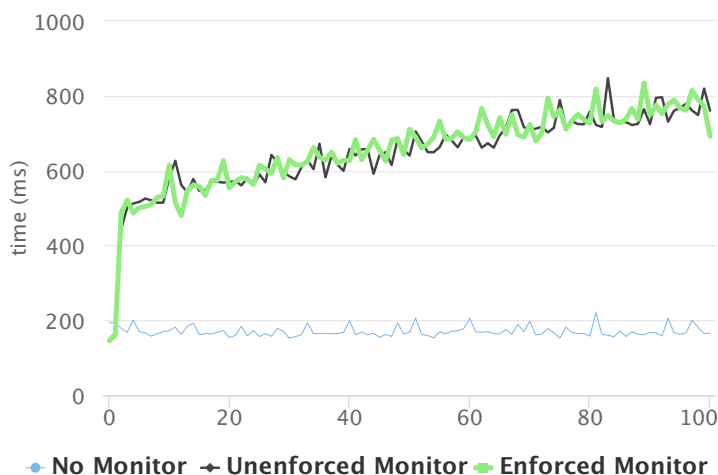
Figure 5.2 – Performance overhead of deploying the monitor
