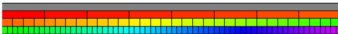
Figure 6.4: Color code used to show our hierarchical segmentation results for a 3-deep tree where nodes in 0-th, first and second layer have respectively 8, 4 and 2 children each. Each node corresponds to a different color of the HSV colormap.
