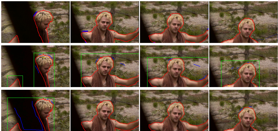
Figure A.3: Comparison with alternative methods on a sequence with occlusions and motion-blur (sequence courtesy of [BWSS09]) First row: Video SnapCut [BWSS09]. Second row: Frame-by-frame GrabCut [RKB04]. Third row: Proposed method. Segmentation results are marked in red. The user interactions, if any, are marked for every frame (Blue: Background seeds, Yellow: Foreground seeds, Green: Bounding box).
