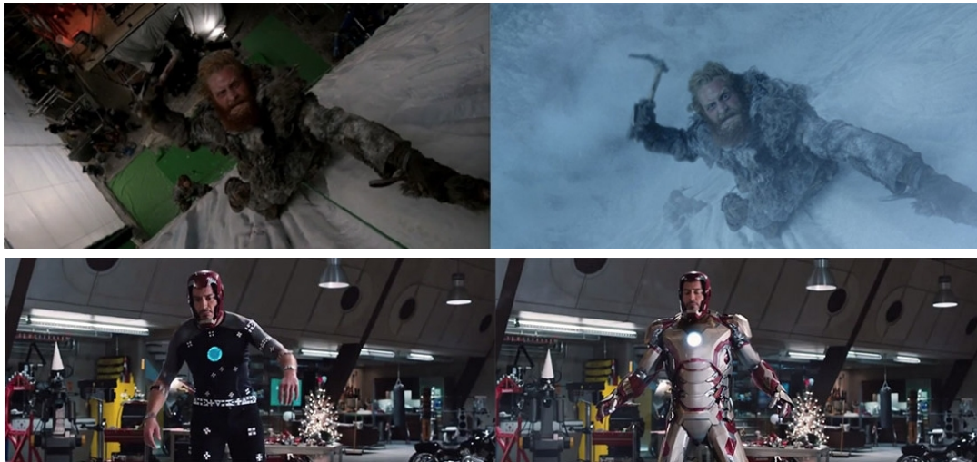
Figure 2.8: Visual effects in film and television industries make strong use of computer vision techniques. Top: Background-foreground separation for blending recorded video with CGI in the acclaimed TV show “Game of Thrones”, by D. Benioff and D. Weiss. Bottom: Motion capture for realistic blending of an animated armor with a real human actor in the film “Iron Man” (2008), by J. Favreu.
