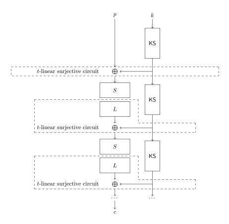
Figure 4.11: Structure of an SPN-Based Block Cipher.
