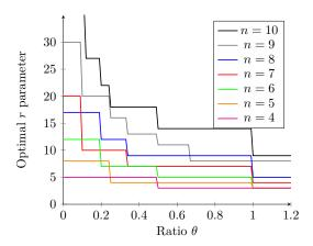
Figure 3.3: Optimal r parameter w.r.t. the CPRR-ISW cost ratio  $\theta$  for  $\lambda \in [4, 8]$ .
