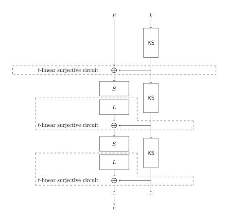
Figure 4.11: Structure of an SPN-Based Block Cipher.
