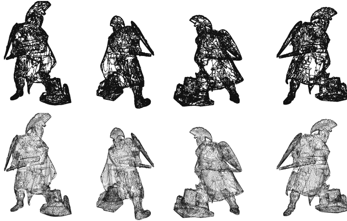
Figure 4.27: “Roman” dataset: 48 silhouettes and projection matrices. Top : Four views of the intersection curves. Bottom : Four views of a point cloud on the visual hull surface (approximately 240000 points).
