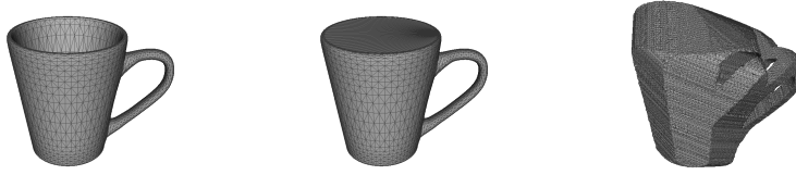
Figure 4.19: An object ( left ), its complete visual hull ( center ), and its finite visual hull associated with four viewpoints ( right ). Note that the finite visual hull is not topologically equivalent to the original object.
