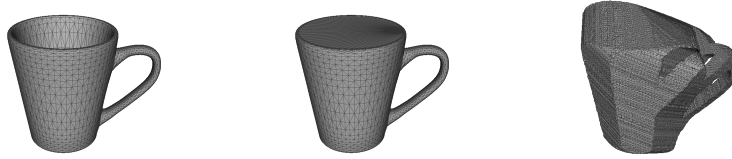
Figure 4.19: An object ( left ), its complete visual hull ( center ), and its finite visual hull associated with four viewpoints ( right ). Note that the finite visual hull is not topologically equivalent to the original object.
