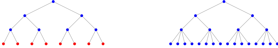
Figure 2.3: An example of approximated tree. The nodes in red are originally associated to arcs; in the approximation, they are replaced by D = 2 nodes containing sample positions extracted from the arcs.
