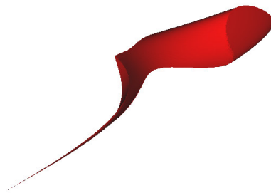
Figure 6.5: Admissible stability region for \gamma , \alpha_1 and \alpha_2 in the construction of Linear-SDIRK schemes of order s + 1 = 10 with 3 additional stages.
