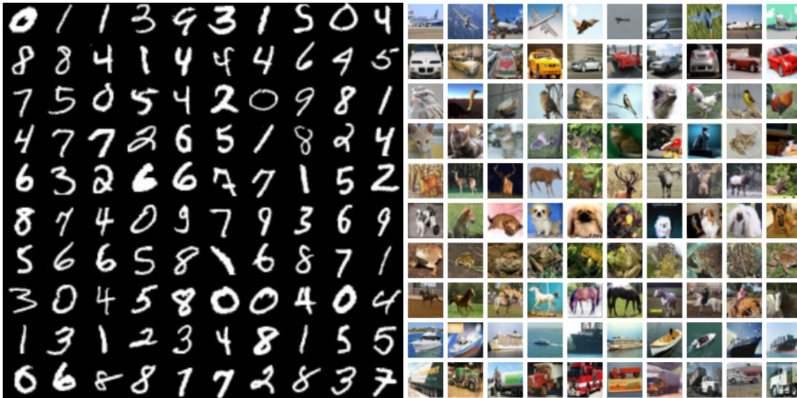
Figure 2-33: Datasets commonly used for neural networks research. Left: MNIST, introduced in LeCun et al. [1998a] , 60000 training examples, 10000 testing examples, 28 \times 28 -pixels binary images, 10 classes. Right: CIFAR-10, introduced in Krizhevsky [2009] , 50000 training examples, 10000 testing examples, 32 \times 32 -pixels RGB images, 10 classes.
