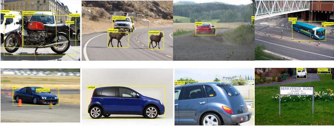
Figure 3-5: Example cars from the Pascal VOC dataset, as well as bounding boxes (in yellow) describing the extent of different objects. The cars appear within complex scenes and at various scales.
