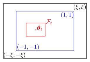
**Figure A.1**: Diagram showing all fields used in the proposed synthetic environment. The robot's field of view (in red) can move within the reachable field (in blue), whereas the participants can freely move within a larger field (in black).
