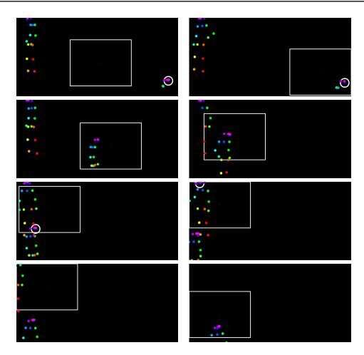
**Figure 3.3**: Example of a simulated sequence used for offline training. The field of view is shown with a white rectangle. Visual landmarks associated with two persons are shown as colored dots. The white circles correspond to simulated speech sources that may correspond to a person.
