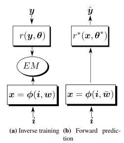
**Figure 4.1**: The method proposed in this chapter performs training by gluing inverse regression (r parameterized by  $\theta$ ) and network fine-tuning ( $\phi$  parameterized by w) in an EM procedure. The parameters  $\theta^*$  of the forward regression  $r^*$  can be derived analytically from  $\theta$ , which allows to predict a target y associated with an input *i*.
