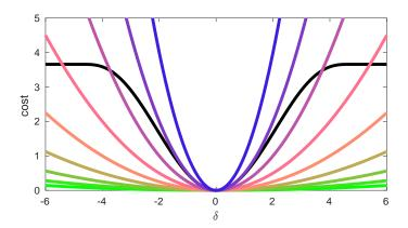
**Figure 5.2**: Cost of the proposed weighted loss (in color) compared to Tukey's biweight function (in black). Different colors represent different values of  $r_n$ , exponentially decreasing from 1 (blue curve, corresponds to classical  $L_2$ ) to  $2^{-8}$  (green curve). Small values of  $r_n$  clearly mitigate the effect of the outlier during the learning of w.
