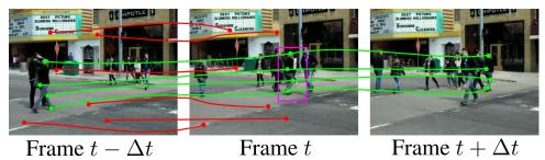
**Figure 2.4**: Trajectory-based description of (pink) bounding-box at frame t: Points of frame  $t - \Delta t$  are densely sampled and tracked up to frame t. At time t, (red) trajectories out of the bounding box are rejected. The remaining end points of trajectories (green) are further tracked until  $t + \Delta t$ . The local space-time area around the green trajectories is then encoded into the individual features  $x_i$ .
