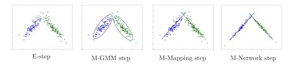
**Figure 4.2**: Training the deep inverse regression EM with a toy example, *e.g.* L = 1, D = 2 and K = 2. The E-step computes the posteriors  $\mu_{nk}^{(i+1)}$ . The M-GMM-step fits a mixture to the data given the posteriors. The M-mapping-step estimates the parameters of the affine regressions (the two lines illustrate the projection of the target space onto the feature space). Finally, the M-network-step fine-tunes the network weights via minimization of a mean-square error loss function.
