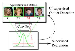
**Figure 5.1**: DeepGUM in a nutshell: the Gaussian-uniform mixture performs unsupervised outlier detection to down-weight the impact of outliers (in red) in the ConvNet loss for supervised deep robust regression.
