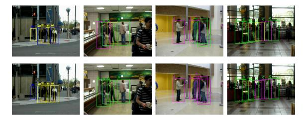
**Figure 2.5**: Example frames from sequences of dataset *A* with single person model (first row) and the proposed model (second row). The color of the box represents the predicted activity (red for *Crossing*, yellow for *Waiting*, green for *Queueing*, blue for *Walking*, purple for *Talking*). On top of each bounding box, the letters show the ground truth activity (*better viewed on screen*)
