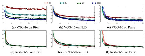
Figure 6.2: Comparison of the training loss evolution with different batch size on VGG-16 and ResNet-50.
