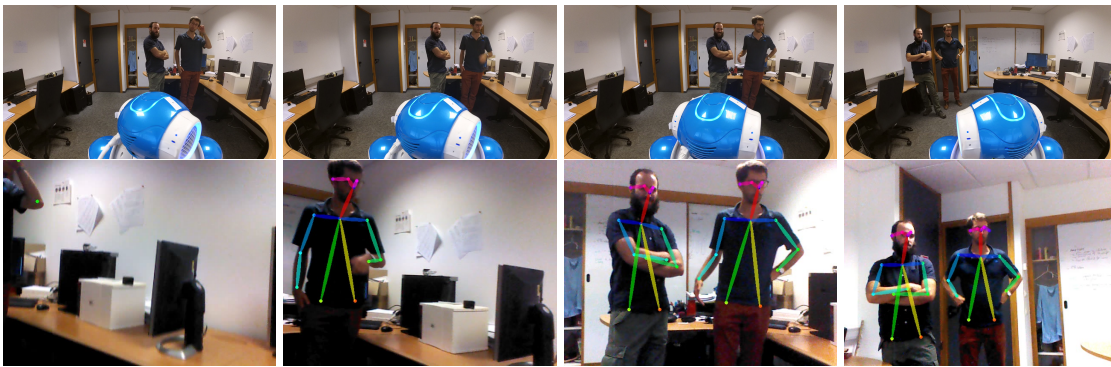
Figure 3.7: Example of a live sequence with two persons. First row shows an overview of the scene, including the participants and the robot. Second row shows the images gathered with the camera mounted onto the robot head. The robot head is first initialized in a position where no face is visible (first column), and the model uses the available landmarks (elbow and wrist) to find the person onto the right (second column). The robot detects the second person by looking around while keeping the first person in its field of view (third column), and gazes the two people walking together (fourth column).
