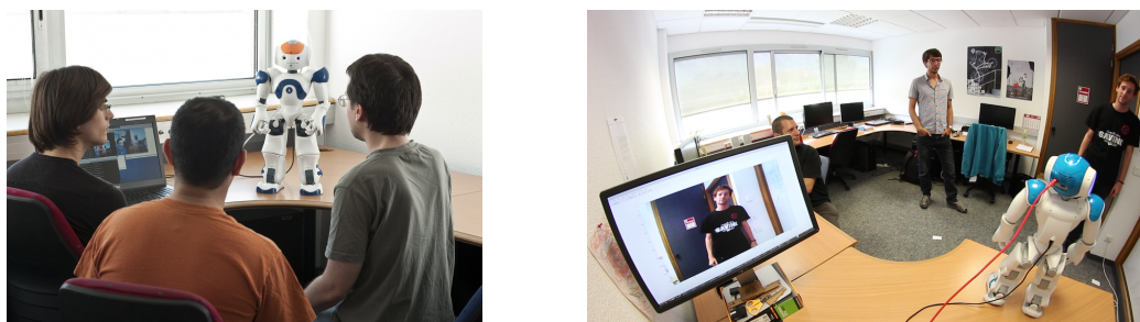
Figure 4.1: A typical scenario in untethered human-robot-interaction. A companion humanoid robot (NAO) perform audio-visual scene analysis in an attempt to detect and locate speakers in the field of view of its camera.
