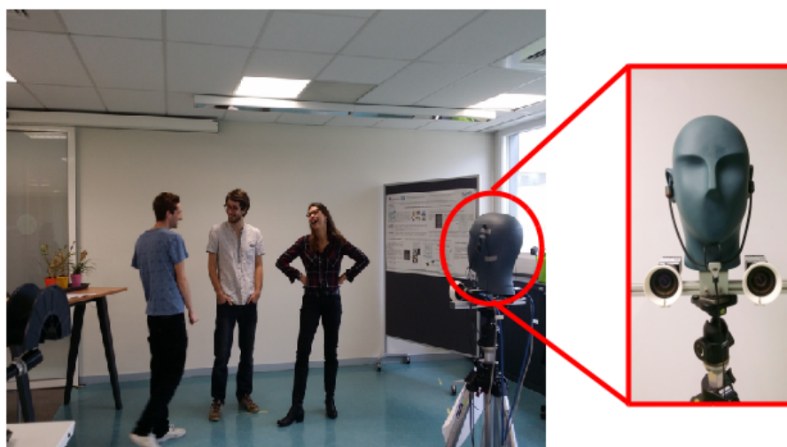
Figure 2.1: A typical scenario in AVDIAR dataset: multiple people engaged in a social conversation. A distant camera-microphone unit circled in red captures the scene globally.
