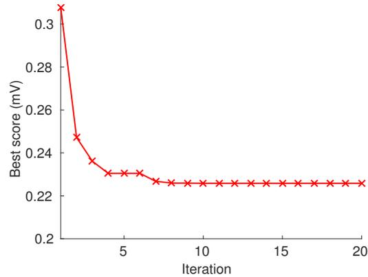
Figure 5.2: Best score versus the number of iterations of the CMA-ES algorithm. The score is identified as the mean error between the simulated and real 12-lead ECG, in mV.
