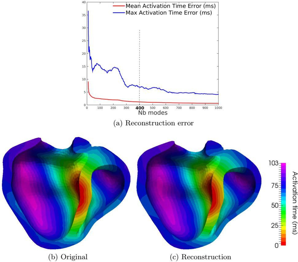
Figure 3.2: Example of reconstruction of an activation map (on 14430 vertices) from the eigenvectors of the stiffness matrix: (a) Reconstruction error wrt. the number of modes (b) original activation map (c) reconstructed activation map from 400 modes.
