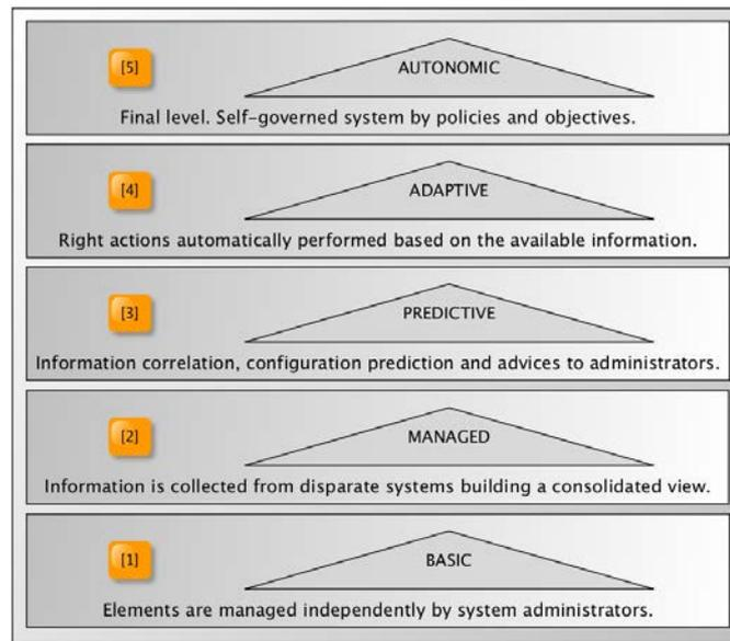
FIGURE 2.2 – Stages towards autonomic computing [82]
