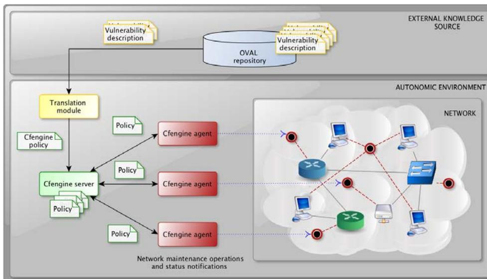
FIGURE 4.3 – High-level architecture
