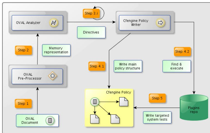
FIGURE 9.1 – Ovalyzer's high-level operation
