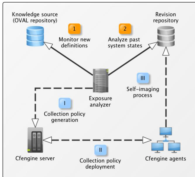
FIGURE 6.2 – High-level imaging and exposure detection process
