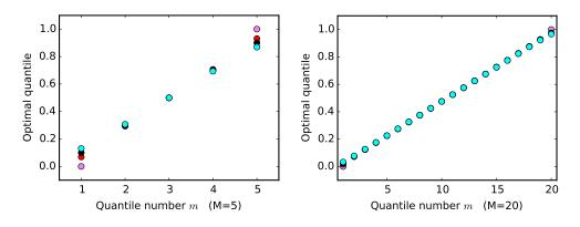
Figure 4.4 – Optimal quantile levels  $F(x_m)$  of the members for M = 5 (left) and M = 20 (right) with weighting functions  $\omega$  belonging to the symmetrical beta family,  $\omega(\alpha) = \alpha^{a-1}(1-\alpha)^{a-1}$ : a = 0 (violet), a = 1/2 (red), a = 1 (black), a = 2 (cyan).
