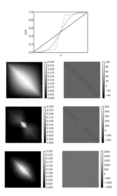
Figure 4.7 – Visualization of R (left) and  $R^{-1}$  (right) in the cases of uniform (top), piecewise uniform (middle) and Gaussian distribution (bottom) for linearly spaced thresholds. The CDFs of the uniform (solid black), piecewise uniform (dashed black) and Gaussian distribution (solid grey) are also shown.
