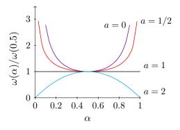
Figure 4.2 – Scaled weighting function  $\omega/\omega(0.5)$  in the symmetrical beta family  $\omega(\alpha) = \alpha^{a-1}(1-\alpha)^{a-1}$ .
