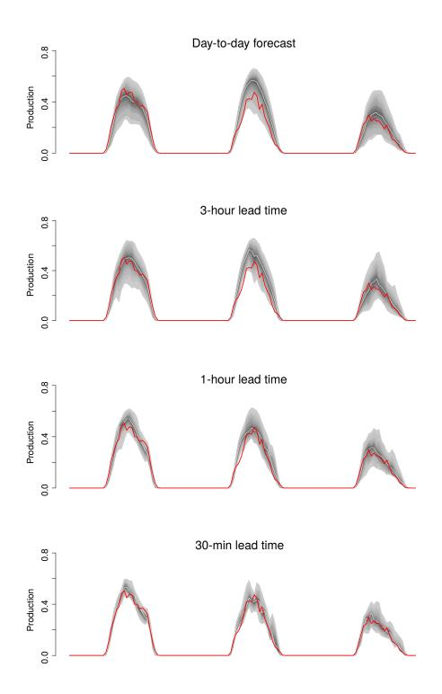
Figure 7.2 – Time series of our weighted probabilistic forecast for 3 consecutive days for Corsica PV production (observation in red). The differences in the time series of intraday lead times of 3 hours, 1 hour and 30 minutes show the evolution of the forecast sharpness and precision. The day-to-day forecast (above) does not benefit from intraday updates.
