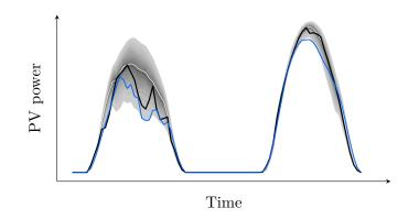
Figure 1.7 – PV production (black), deterministic forecast (blue) and probabilistic forecasts (confidence intervals in shaded gray, median in white) for two consecutive days.
