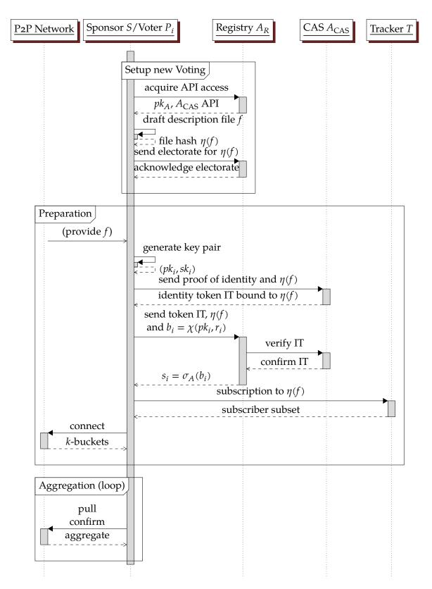
Figure 6.1: ADVOKAT-Vote sequence diagram. The steps of the sponsor *S* to setup a new voting and the consecutive preparation of every voter  $P_i$  is given. The authorities  $A_R$  and  $A_{CAS}$ , and the tracker *T* are not required any longer afterwards.
