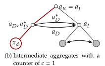
Figure 5.3: Detecting dishonest peers in ADVOKAT. Two scenarios are considered with honest peers computing aggregates  $a_i$ , respectively  $a_I$ , and one dishonest peer  $P_d$  at leaf node  $x_d$ . Arrows indicate pull requests. In can be shown that in all considered scenarios, attempts of  $P_d$  to introduce manipulated initial aggregates  $a_d^*$  or intermediate aggregates  $a_D^*$  can be detected.
