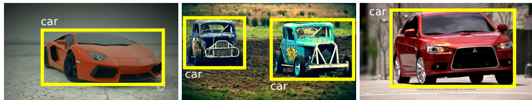
Figure 1.5: Example of intra-class variations, where three instances of the same object class car have very different appearance: different car models, shapes, colors, etc. Examples from the YouTube-Objects [Kalogeiton et al., 2016; Prest et al., 2012a] and ILSVRC VID 2015 [Russakovsky et al., 2015a] datasets.
