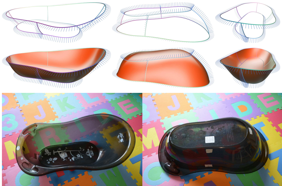
Figure 5.15: Baby bathtub acquired with Morphorider. Scanning this translucent object was not an issue.
