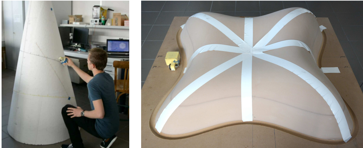
Figure 5.4: Physical surfaces used as ground truth in our tests: cone ( left ) and lilium ( right ).
