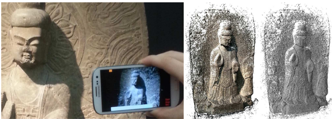
Figure 1.5: Reconstruction of a Shakyamuni Buddha statue (height: 1.6 meters) using a smartphone. Image from [Tan+13].
