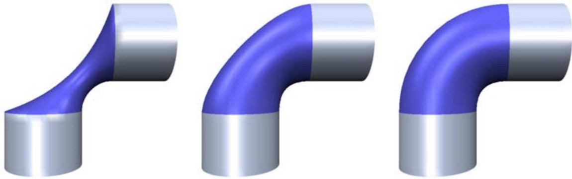
Figure 4.2: The framework of Botsch and Kobbelt [BK04] enables prescribing different levels of continuity. The three pipes were obtained by solving \Delta^k \mathbf{v} = \mathbf{0} , k = 1, 2, 3 , with C^{k-1} continuity on the boundary. Image from [BK04].
