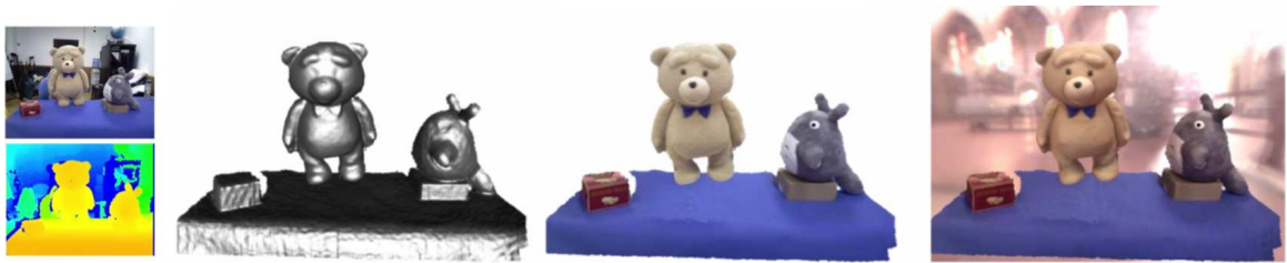
Figure 1.3: Real-time scene reconstruction using a single RGB-D camera. Image from [Guo+17].
