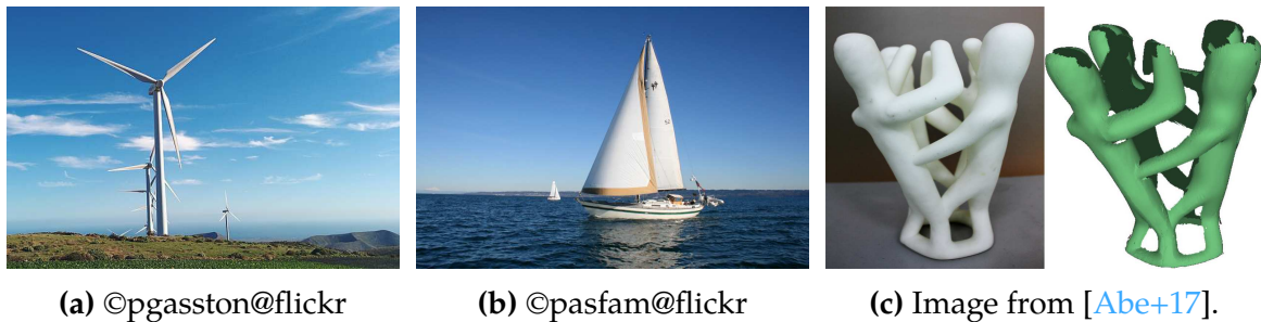
Figure 1.6: Issues of optical scanners. (a-b) Traditional 3D scanning methods cannot be used with large, inaccessible, moving and/or deforming objects. (c) Optical scanner reconstruction of a self-occluding object with high genus fails to recover the interior part.
