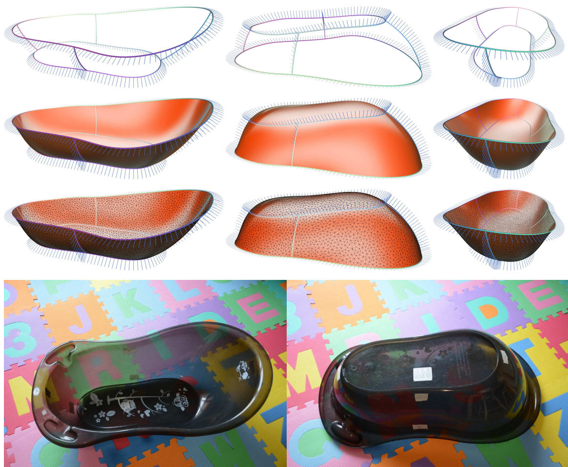
Figure 5.15: Baby bathtub acquired with Morphorider. Scanning this translucent object was not an issue.
