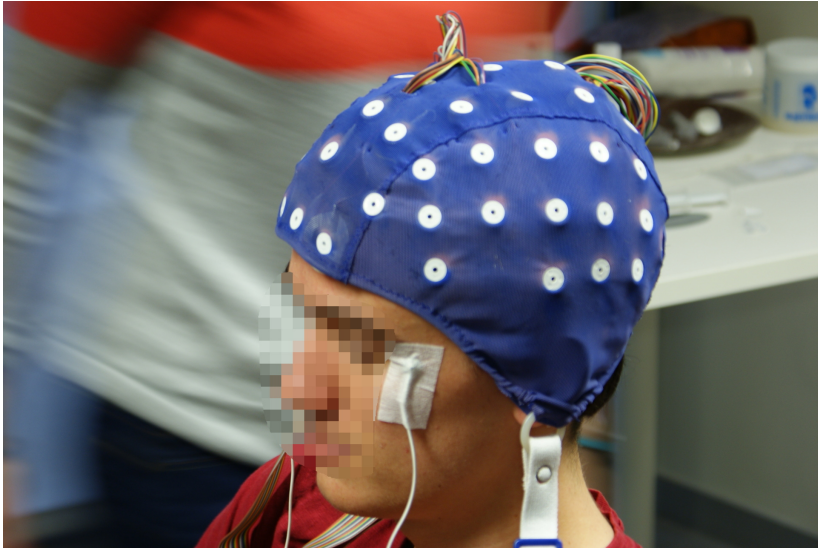
Figure 2.1: EEG cap placement using wet based electrodes.
