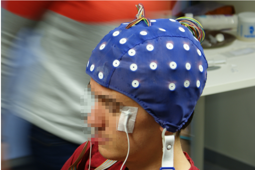
Figure 2.1: EEG cap placement using wet based electrodes.
