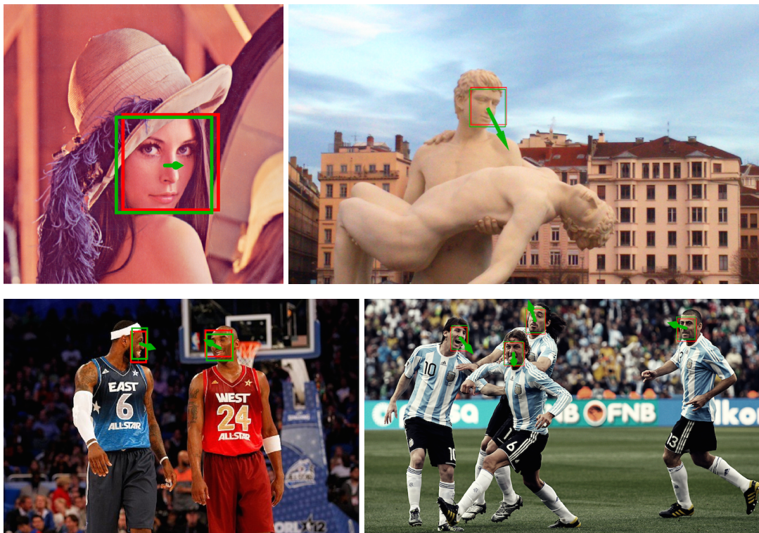
Figure 2.6: Examples of simultaneous estimation of head-pose angles and of bounding-box shifts. The initial bounding box (found with an automatic face detector) is shown in red. The estimated bounding box is shown in green.
