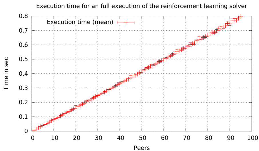
Figure 4.6: Execution time for the reinforcement learning solver in relation to the number of peers.
