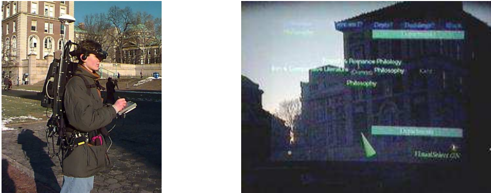
Figure 1.21: Touring Machine system overlays AR information in outdoor environments.
