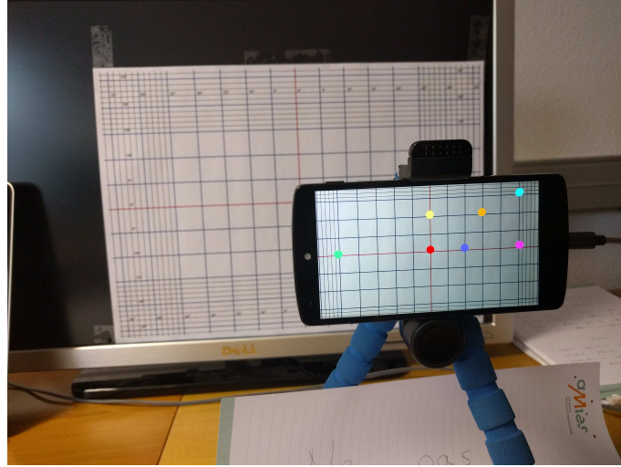
Figure 5.7: Virtual spheres placed at a predefined position on a custom target to verify FOV.
