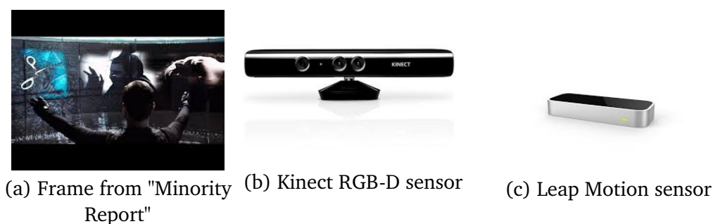
Figure 1.1: (a) – frame from "Minority Report" movie presenting computer interface controlled by gestures, (b) and (c) sensors which are used in modern human computer interfaces.
