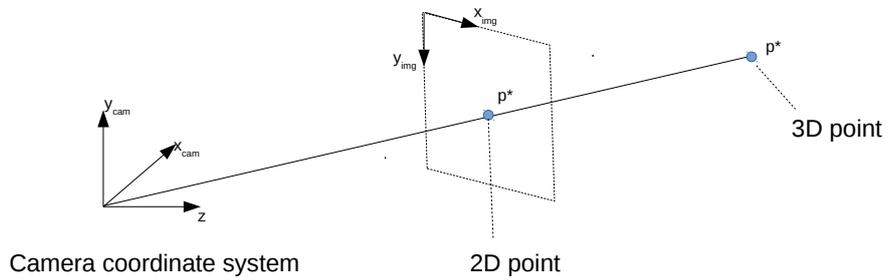
Figure 4.2: This figure shows graphically, the relation between 2D point  $p$  obtained from RGB detector that is defined in an image coordinate system and  $p^*$  3D point defined in camera coordinate system.
