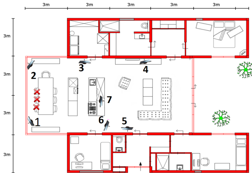
Figure A.1: Plan of the apartment where Smarthomes dataset was recorded. Numbers indicate Kinect sensors locations.
