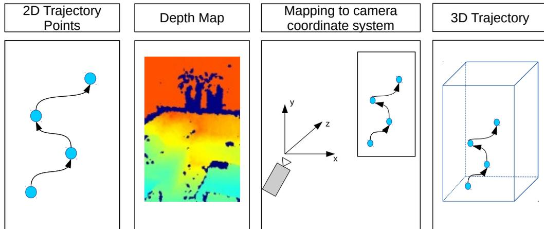
Figure 4.1: This figure shows the steps to obtaining 3D Trajectory points. First 2D trajectories based on RGB image are obtained. Then depth-map is processed with median filtering. In third step 2D points are transformed to 3D camera coordinate system, image  $x_{img}, y_{img}$  positions,  $z$  from depth-map are transformed using pinhole camera model. In the last step 3D points are stacked together to form trajectory.
