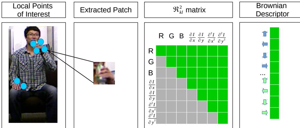
Figure 6.3: Brownian Descriptor is created by taking upper half of *distance correlation*  $\mathcal{R}^2$ .
