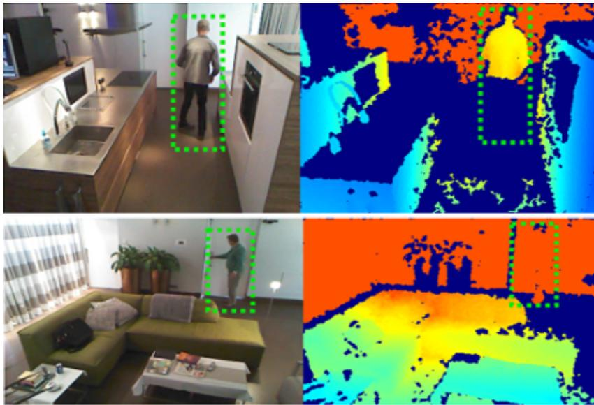
Figure A.2: Depth map quality in Smarthomes dataset. Dark blue color indicates missing depth values. Depth value is not available for a floor and a kitchen workspace, also depth information cannot be measured on black jeans (top row). In the bottom row person is too far from the sensor.
