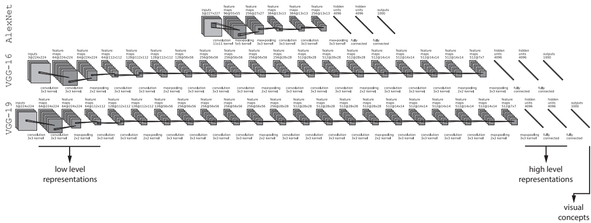
Figure 2.11: Three popular convolutional neural network architectures: AlexNet, VGG-16 and VGG-19. Regardless of number of layers the initial convolutional layers provide good low level image embeddings, the fully-connected layers towards the end of the architecture provide good high level embeddings and the last, output layer, provides visual concepts.
