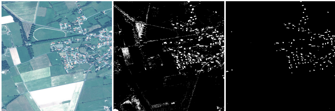
(a) Color pansharpened input (b) SVM on individual pixels (c) FCN (two resolutions + fine-tuning)
